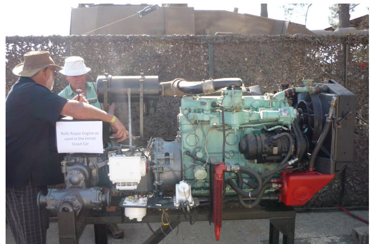
Rolls Royce engine and gearbox and final drive as used in Ferret Scout Car
