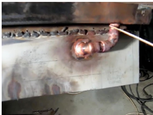
Figure 2 - Drainage from tyre well now drains through the new inner panel
