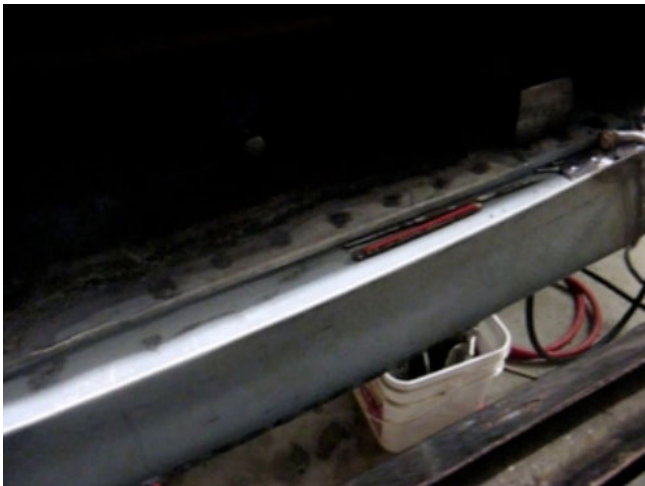
Figure 7 - The joint between the tyre door and the body which had no weather seal
