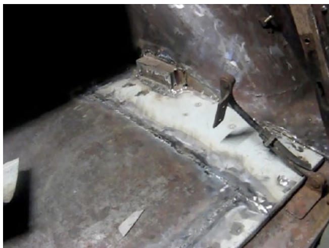
Figure 1 - Tyre well floor straightened and repaired
