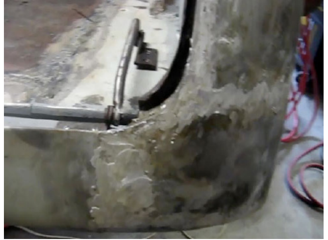
Figure 6 - Welds on corner panels lead wiped
