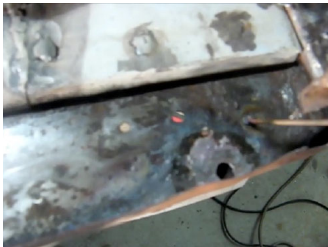
Figure 3 - Drain hole in tyre well floor enlarged
