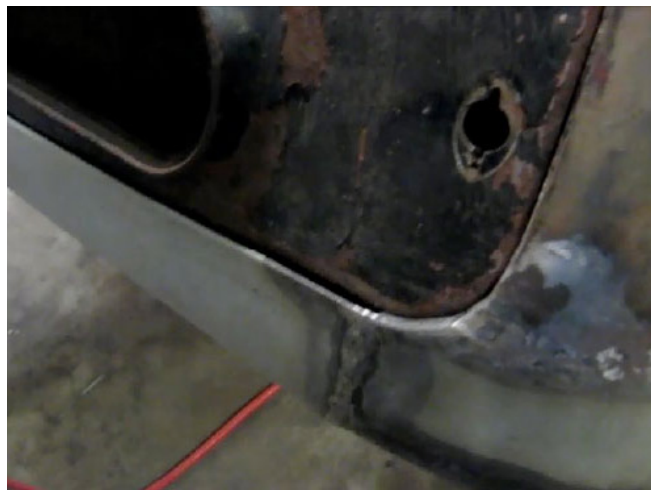
Figure 4 - Outer panels fabricated and welded in place
