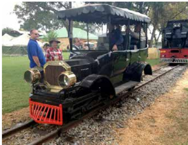
Retrofitted with a Toyota diesel engine and gearbox
