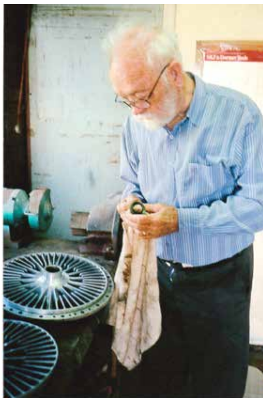
“Doctor” Stan Richards performing open heart surgery on Lynden Braye’s Conquest fluid flywheel
