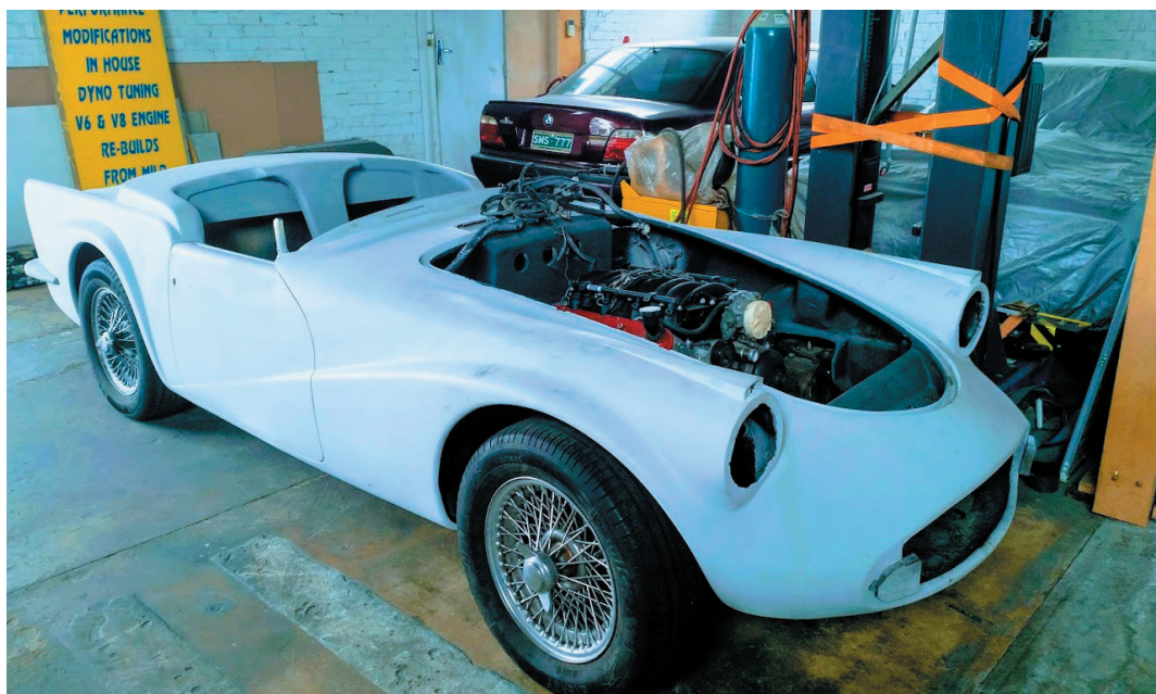
Discovery of a long lost SP250, note body mods including nose, scuttle, mudguard sweep and hood recess cover
