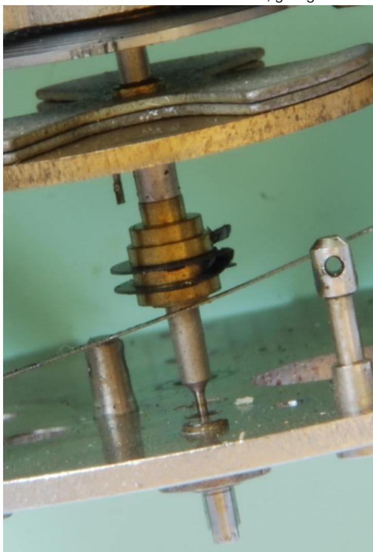
Catching blades – note the pin on the wheel. Other gears removed in this picture.
