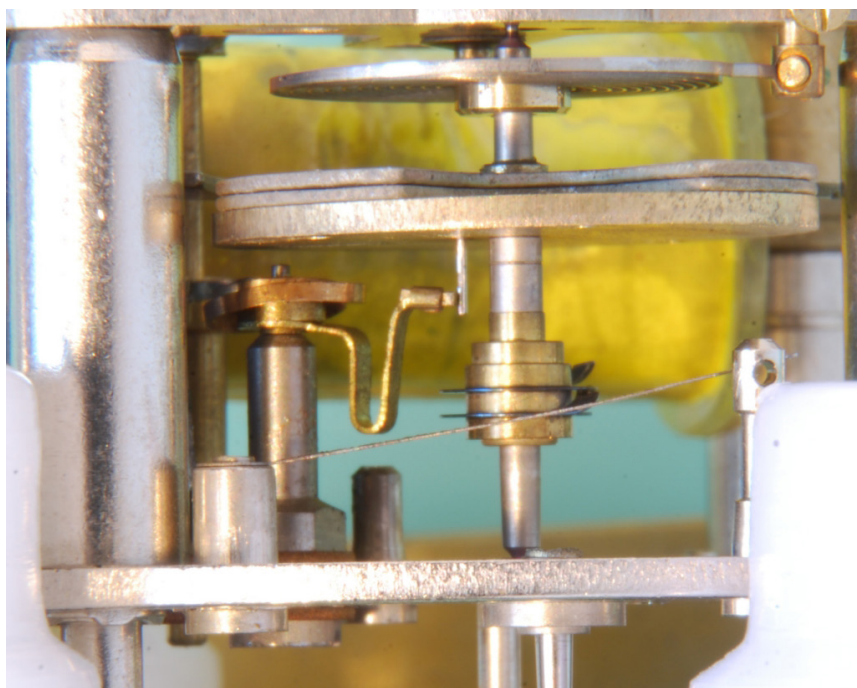
The pin and sprung contact, in original form.
