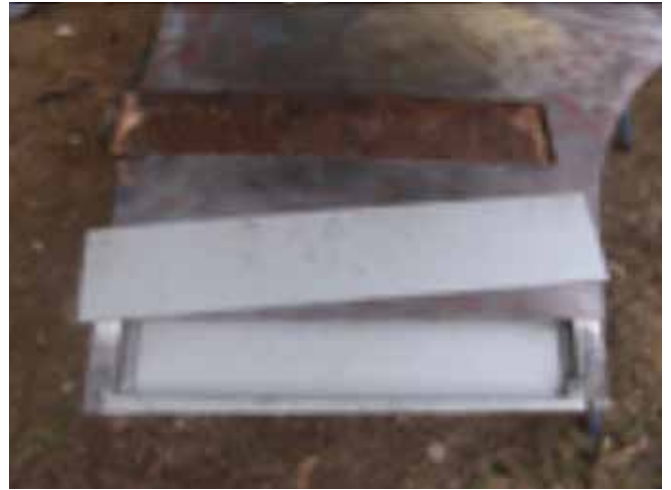
Figure 4 - Repair section for the door skin ready for welding
