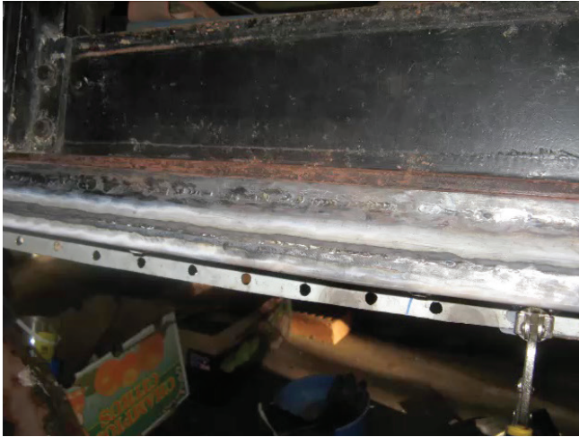
Figure 7 - Bottom sill ready for plug welds to inner sill
