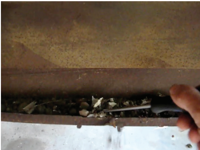
Figure 8 - Passenger inner sill removed showing internal debris
