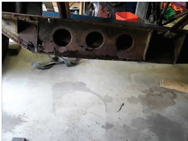
Figure 1-Inner drivers sill rusted through
