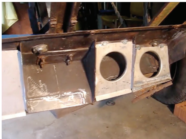
Figure 3 - Central pillar support repaired new inner sill at rear
