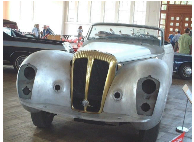
Above: Photos of Mr Hamatto's GG stripped down to the bare metal, awaiting restoration at the workshop in Czechoslovakia.
