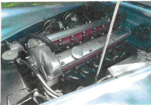
120 Engine: The legendary 3.4 litre XK engine, this variant on twin 1½" SUs.
