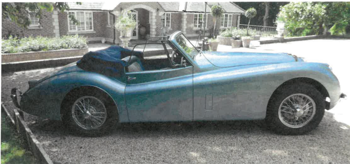
The XK120, like the Barker, has a beautifully lined, easily erected hood that sits relatively neatly on the rear tonneau panel when folded.
