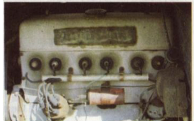
His overhead-valve six-cylinder 2565cc engine
