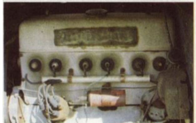
His overhead-valve six-cylinder 2565cc engine
