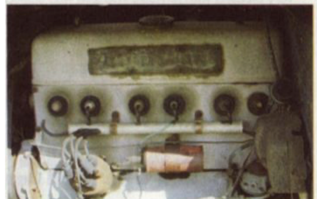
His overhead-valve six-cylinder 2565cc engine
