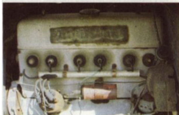
His overhead-valve six-cylinder 2565cc engine
